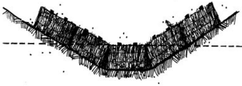
Location of Straw bale barrier in swale section view
