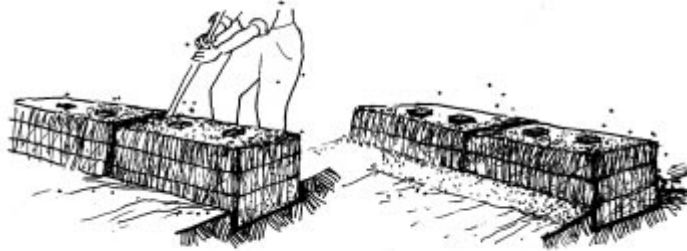
Location of Straw bale barrier in swale section view
