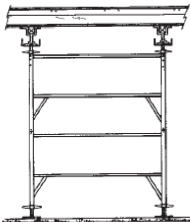
Typical Shoring Tower with Stringers, U-Heads
