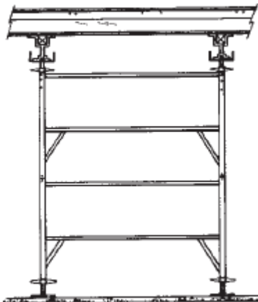
Typical Shoring Tower with Stringers, U-Heads
