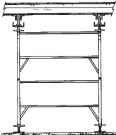
Typical Shoring Tower with Stringers, Adjustable Base Plates, and U-Heads
